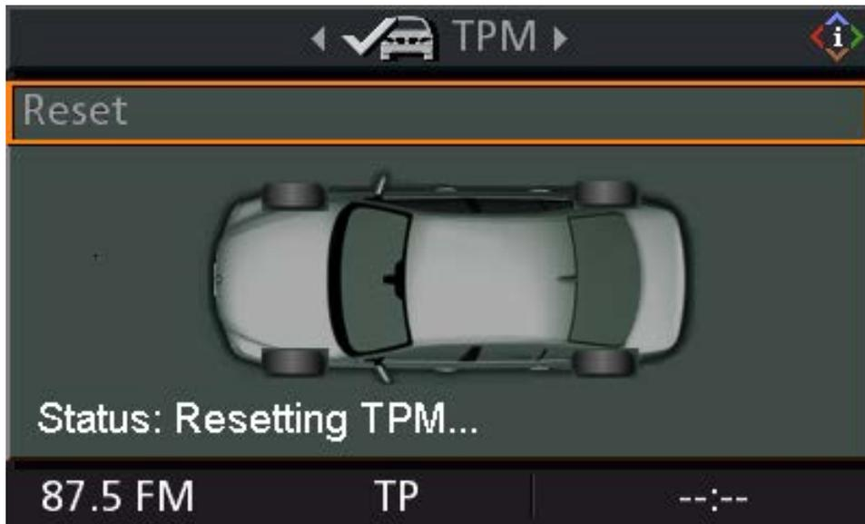
In order for the reset procedure to be completed, the tires must be at the minimum allowable pressure which is approximately 1.4 bar (20 psi) to 1.6 bar (23 psi). If the tire pressure is too low, the system will not complete the reset procedure. When complete, the control display will switch to “Status” TPM active” and the tires will switch to green.
