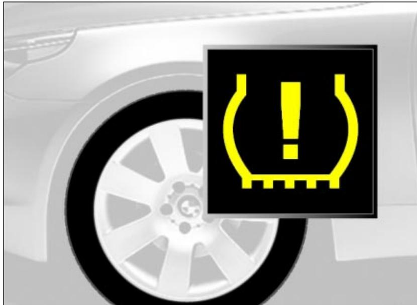
In addition to safety issues, under-inflated tires can cause a reduction in fuel economy and overall tire life. Studies by tire manufacturers have shown that tire life can be reduced by 50% when the tires are under-inflated by as little as 20%.
