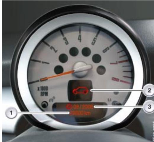
The upper display (#2) in the tachometer is lit up by a symbol (e.g. an oil can symbol for an oil change).
