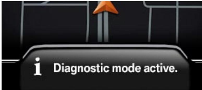
Wait a few seconds until the other indicator lights have gone out. Next, press and hold the BC button on the turn signal/high beam stalk until the first service job appears in the display.
