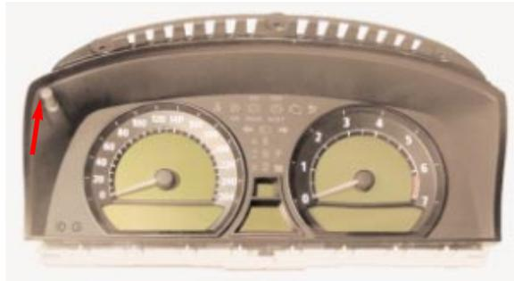
The service menu appears in the speedometer and tachometer.
