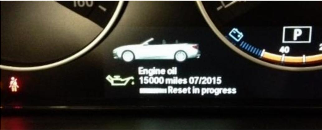
The reset of the service is completed when the status reads "Reset Successful".
