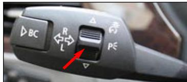
Press and release the BC button when the desired service has been reached. The word "RESET" will appear on the display.
