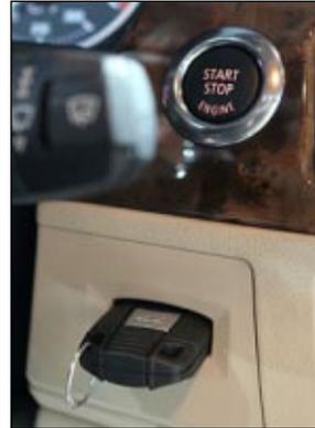
3. Press and hold the central lock button **(in the center of the dash panel)** in the unlock position, and then press the start/stop button (to activate KL-15) while continuing to hold the unlock button.
