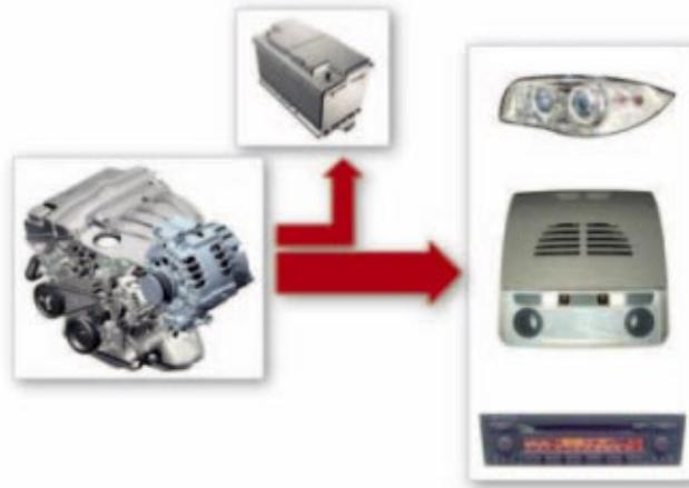
The task of the vehicle electrical system is to provide electrical energy for the vehicle and all its functions. Priority is given to maintaining the starting capability of the vehicle. The purpose of the energy management system is to ensure and balance the energy in the vehicle under all operating conditions.
