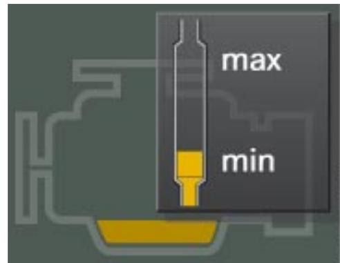
If the oil level drops below minimum, the graphic appears with a red oil sump and an oil dipstick that represents the low oil level in red.
