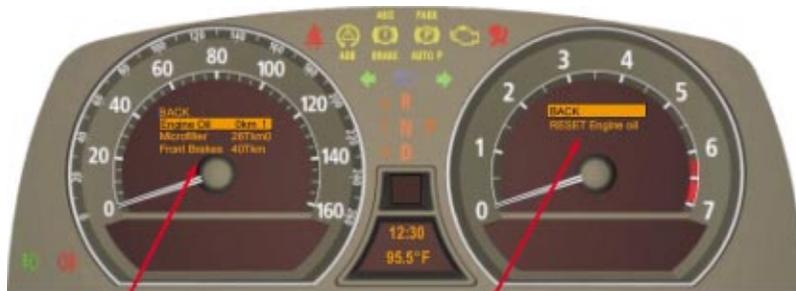
The service menu can be scrolled through by pressing and releasing the reset button. Once the desired item for service is to be reset, press and hold the reset button. Press and hold the reset button again once the sub menu is active to reset the service. To exit the service menu, scroll to the BACK selection on the display and hold the reset button.
