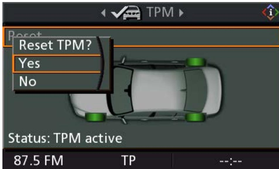
Once the reset mode is initiated, the vehicle must be driven in order to complete the process. This is to ensure that there is no RAF interference or erroneous signals from other vehicles which use similar TPM system components.
