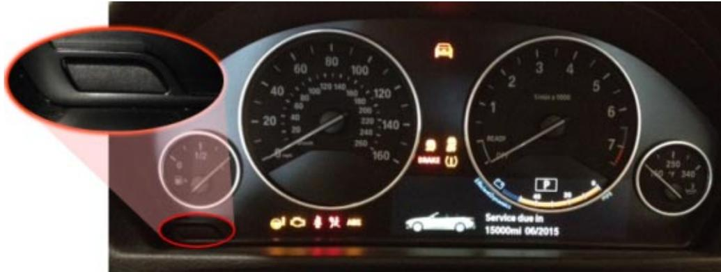
It is possible to scroll through the different service items, by releasing the button and pressing it again until the desired service is reached.
