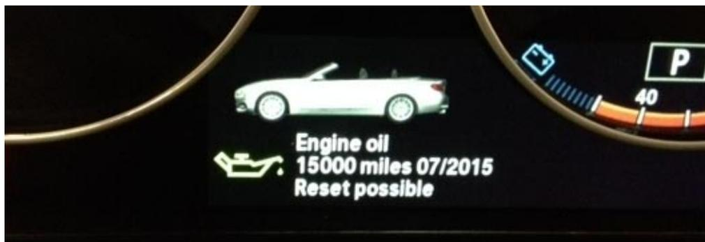
Confirm the reset procedure by releasing the button and then pressing it again for 3 seconds.
