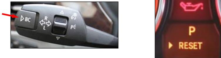
Press and hold the BC button on the desired service to reset. The reset takes place when the clock appears next to the "RESET" display. The reset is then complete.
