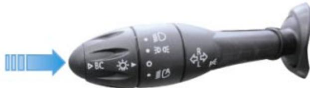
To reset, press and hold the on-board computer button until the word "RESET" appears in the lower display.
