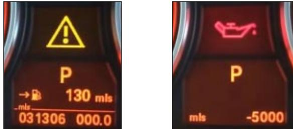
It is possible to scroll through the different service items, by releasing the cluster button and using the scroll feature on the BC stalk until the desired service is reached.
