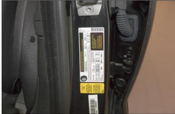
As per BMW Group guidelines, the tire pressure should be checked regularly. The owner's manual states at least twice a month and prior to any long trips. Tire pressure information can be found on the tire pressure placard on the b-pillar. There are also tire pressure charts in the owner's manual as well.
