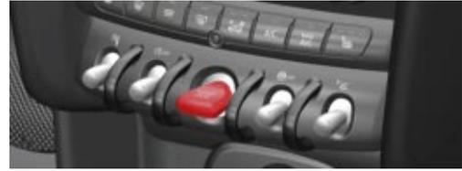
Press and hold the trip reset button until the 1st maintenance service appears in the LCD display.
